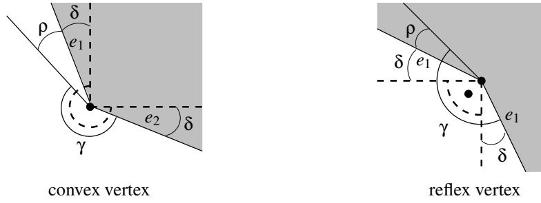
Figure 2.9: Maximal deviation from the outer angle ( \gamma ) and the assumed (dashed) angle for a convex or reflex vertices.
